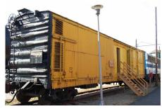
from hatches in the roof. Rock salt would be added with the ice to lower the temperature. The cold would move out through holes in the bunker to keep the food cold. There were tracks in the ceiling to hang meat hooks and sides of beef or hogs. Wooden pallets would be
